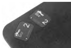
View C PSPs ready for Scanning
