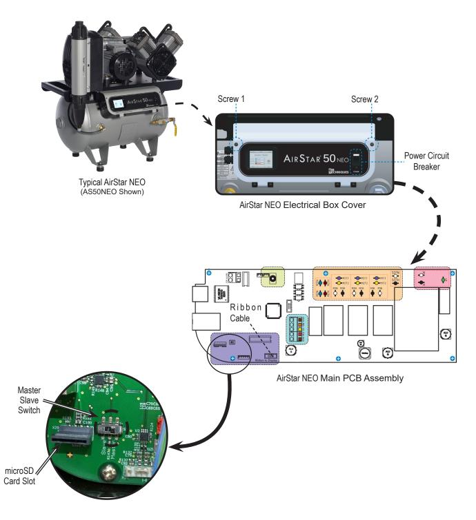
Figure 5. Tandem Compressor Connection
