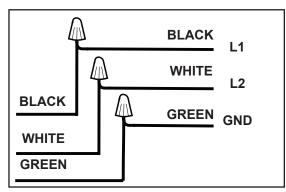
Figure 3. Electrical Connection Box
