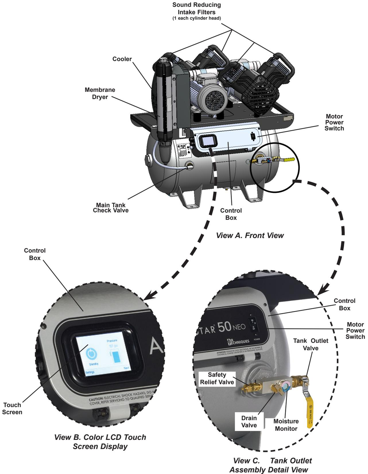
Figure 1. AirStar NEO Parts Location
