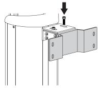
• Push the device to the intended position on the wall. A minimum distance of 28 inches (70 cm) o
