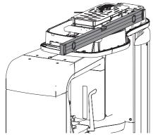
• Insert a M12x15 screw on the back of the telescopic column and hence align the device.
