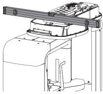
• As required, screw in the corresponding screws and hence align the device.
