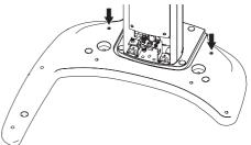
• Attach the stand cover with three M5x8 screws.
