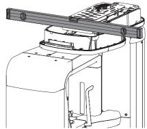
• Use a spirit level to align the device lengthways.
