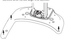
Use a spirit level to align the device lengthways.
