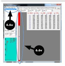
v. Observe the red area around the collimator. If the area to the left or right of the collimator is ≤1 pixel, repeat the exposure.
