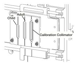
4 Continue to adjust the collimator using the AISU tool until successfully calibrated.
