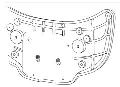
• Tighten the stand using two M10x20 screws.
