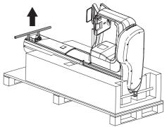
Screw two M10x30 screws into the adapter plate.
