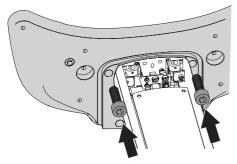
• Tighten the two screws under the stand.
