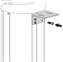
• Mount the wall holder on this bracket with two M8x20 screws and two nuts. Do not tighten the screws yet.
