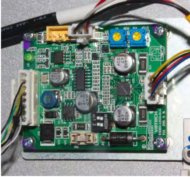
Fig. 138 Board for controlling the X-ray positioning beam for the Frankfort horizontal
