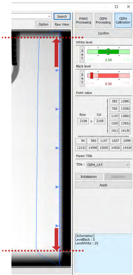
Fig. 169 Alignment of the left and right-hand edges on the blue grid line
