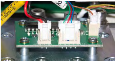
Fig. 141 Board for control of the X-ray alignment
