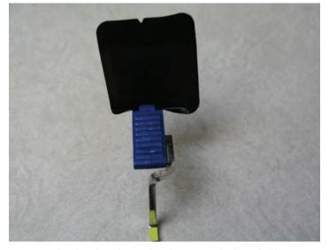
Figure 2—The phosphor plate is placed into a standard XCP holder (DENTSPLY Rinn).
