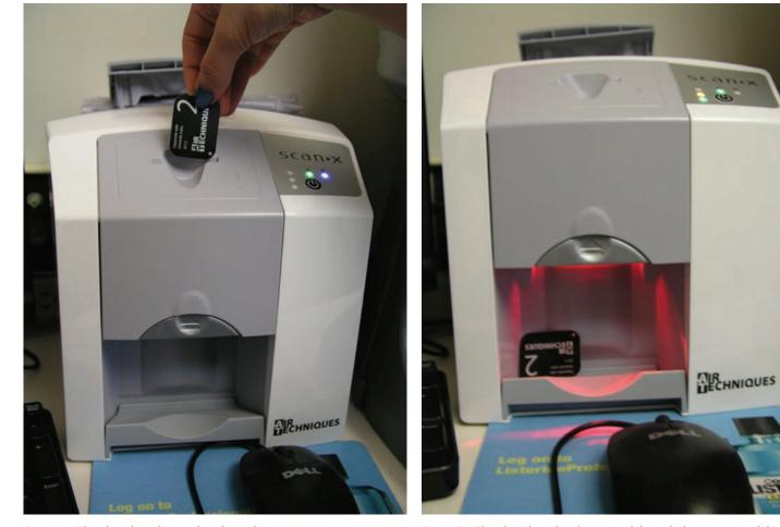
Figure 6—The phosphor plate is placed into the scanner.
