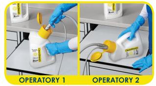
Operatory 1: Place Dispenser in upright position. Attach hoses, open handpiece valves, aspirate 1 liter per operatory (stops automatically after 1 liter is aspirated; no monitoring needed)
