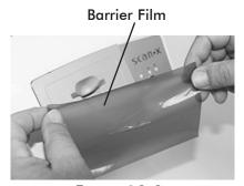
Figure 13-2. Applying barrier film
