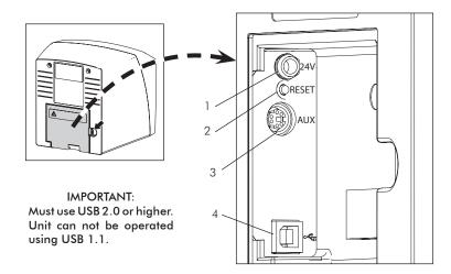
Figure 10-1. ScanX Swift Rear Panel Connection Ports
