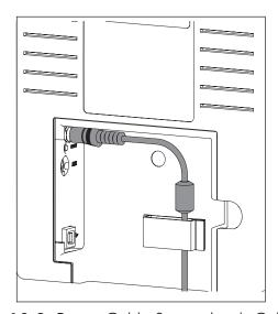
Figure 10-3. Power Cable Secured with Cable Clip
