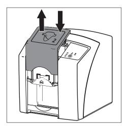
Figure 14-2 Inlet Guide Cleaning
