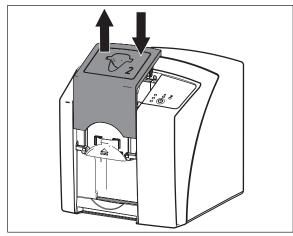
View B. Lift and remove the inlet guide.
