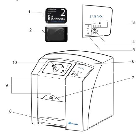
Figure 6 -1. ScanX Swift Controls and Indicators
