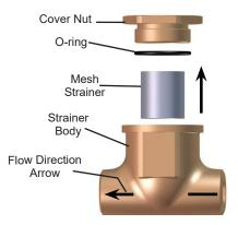
Figure 13. Water Inlet Strainer Location
