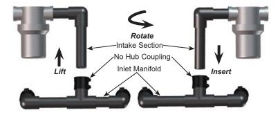
Figure 6. Changing VacStar 50 and 80 NEO Operatory Suction Connection Side
