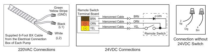
Figure 9 VacStar NEO Electrical Connections
