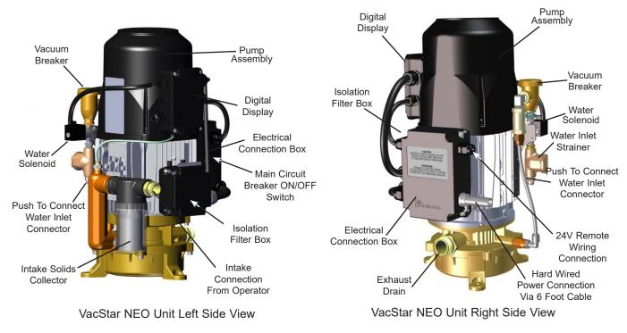
Figure 2. VacStar 20 and 40 NEO Parts Location
