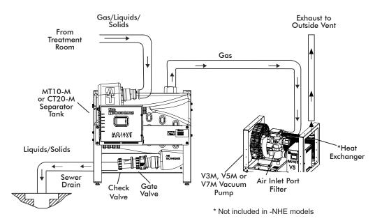
Figure 2. Typical MOJAVE Functional Flow Diagram
