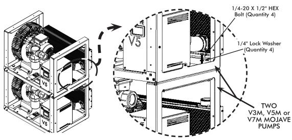
**Note:** See MOJAVE V3M, V5M and V7M Pump Accessory Pack, P/N H5170 or H5307, for required fastener hardware. Remove leveling feet from pump or tank to be stacked.
