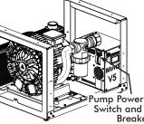
ump Power On/Off Switch and Circuit Breaker
