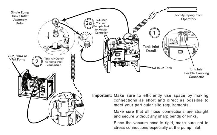
Figure 9. MOJAVE V3M/V5M/V7M Pump and MT10-M Tank Connection Diagram, Sheet 1
