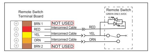
Important: Terminals BRN 1 & 2 are not used when making the 3-wire connection.
