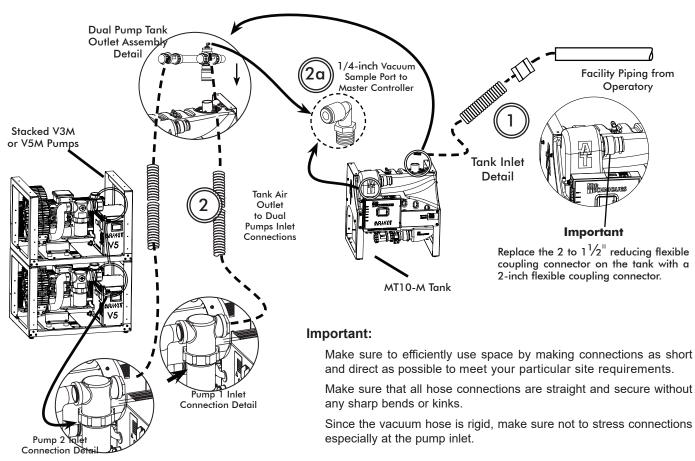
**Note:** If more than 15 feet of the 1/4 inch OD Urethane Tubing is needed, order P/N 51453 for additional 15 foot lengths.
