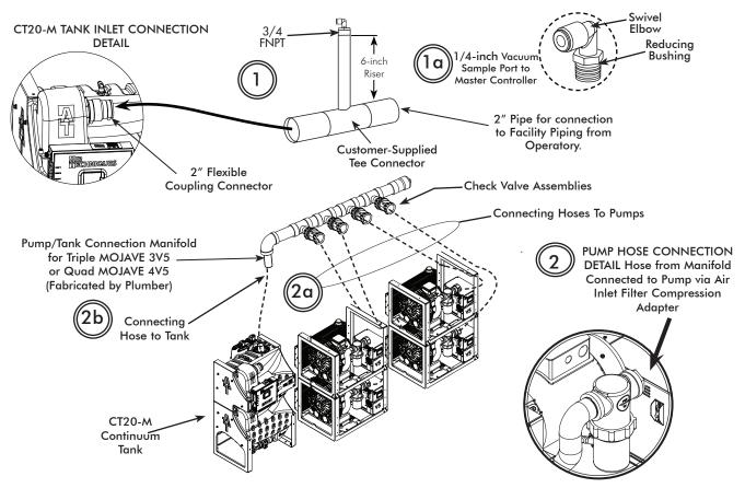
Figure 12. 3V5M or 4V5M System Connection Detail Using Accessory Kit
