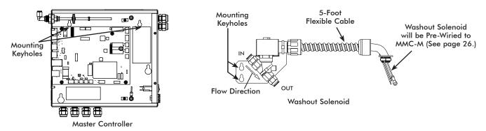
Figure 8. MOJAVE Master Controller and Washout Solenoid Optional Mounting
