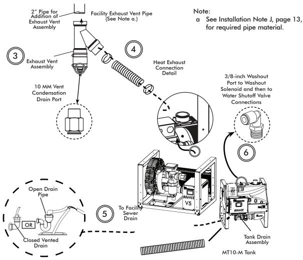
Figure 9. MOJAVE V3M/V5M/V7M Pump and MT10-M Tank Connection Diagram, Sheet 2
