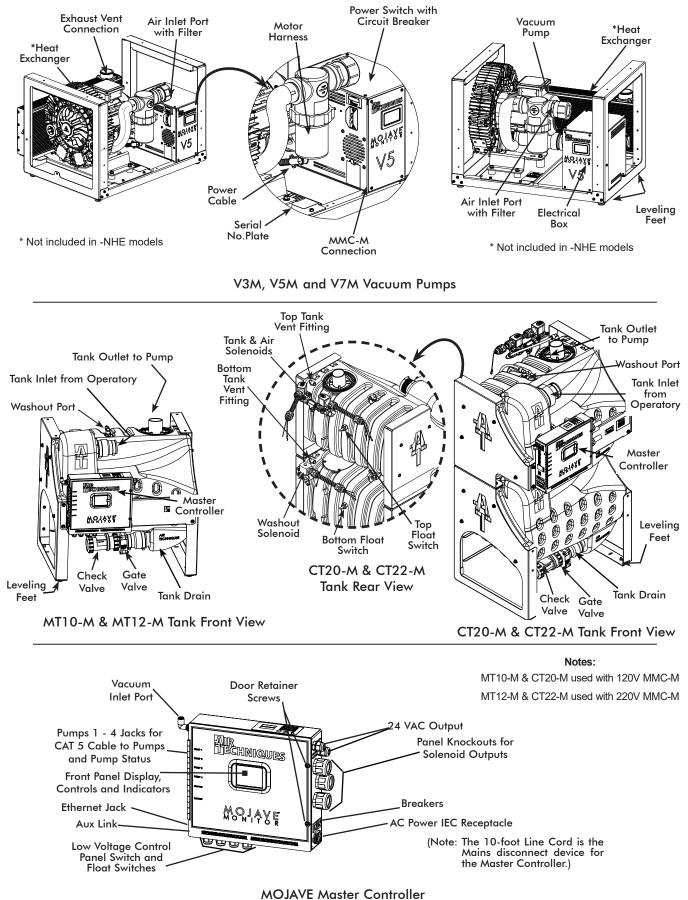
Figure 1. Main System Components
