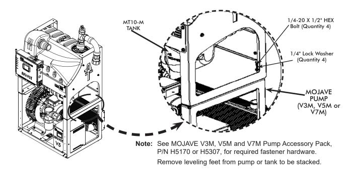
Figure 6. Stacking the MT10-M Tank on Top of a MOJAVE Pump Hardware Detail
