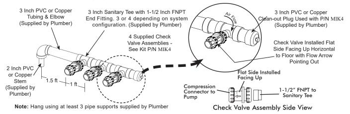
Figure 11. Pump/Tank Connection Manifold Fabrication
