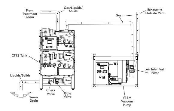
Figure 2. Typical MOJAVE Functional Flow Diagram
