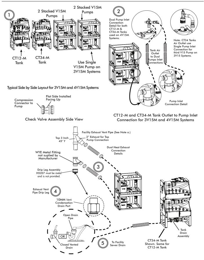
Figure 13. CT12-M and CT34-M Tank Output, Drain and Pump Vent Connection Diagram
