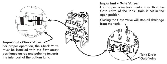
Figure 7. CT12-M and CT34-M Check Valve and Gate Valve Operating Position
