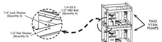
Note: See MOJAVE V15M Pump Accessory Pack, P/N H5403, for required fastener hardware. Do Not install leveling feet on top pump to be stacked.
