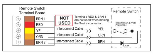
View B. 3-WIRE GREEN INDICATOR ONLY 24 VDC REMOTE SWITCH INSTALLATION
