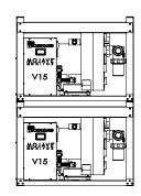
2V15M System Installation: Two V15 Pumps Stacked with One CT12-M Tank on the Side
