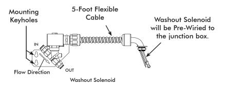
Figure 8. Washout Solenoid Optional Mounting
