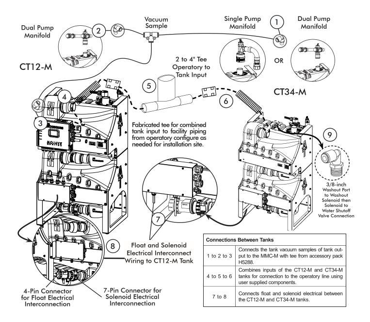
Figure 14. CT12-M Tank to CT34-M Tank and Washout Port Connections Diagram
