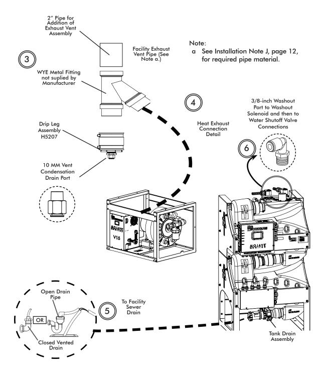
Figure 10. MOJAVE V15M Pump Vent and CT12-M Tank Drain Connection Diagram
