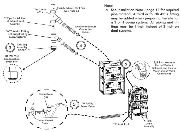
Figure 12. MOJAVE Dual Pump Vent and Tank Drain Connection Diagram
