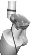
Adjust the X-ray parameters (kV, mA, s) on the X-ray unit (use the maxillary molar settings, see "14 Recommended exposure times") and trigger an X-ray image acquisition.
