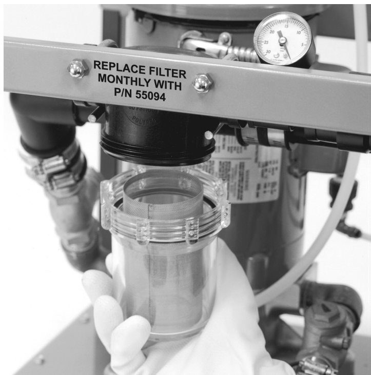
Figure 12. Intake Solids Collector Location
