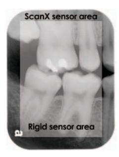
**ScanX Swift's** flexible phosphor sensors can offer 17% to 38% more image area than direct sensors.
