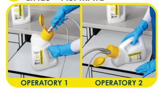
**Operatory 1:** Place Vortex Dispenser in upright position. Attach hoses, open handpiece valves, aspirate 1 liter per operatory (stops automatically after 1 liter is aspirated; no monitoring needed)
