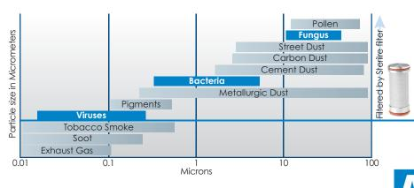
\*AirStar Bacterial filters are used in conjunction with the Membrane Drying unit and have been independently tested by the SGS Frisenius Institute showing a retention of greater than 99.99995% for particles smaller or equal to 0.01 micron in size, as well as a retention of greater than 99.994% using test virus PHiX174. AirStar Bacterial filters are in compliance with ULPA U16 according to 1822-1:2009.
