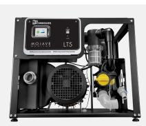
sound-reducing impeller design, a 3-phase motor that generates higher torque and less heat, and extended heat-resistant motor bearings. All wetted metal parts are nickel plated or stainless steel. It also has an aluminum high-performance air-exhaust heat exchanger and a rugged metal chassis.
