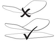
Do not scratch the phosphor storage plates. Do not subject the phosphor storage plates to pressure from hard or pointed objects.
