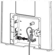
> Plug the mains plug into the power outlet.
