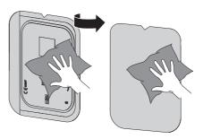
Allow the barrier envelope and phosphor storage plate to dry completely.
