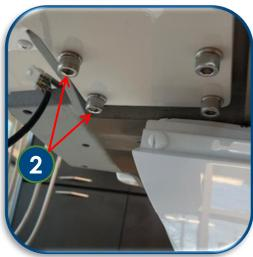
NOTE: without the 3/4" bracket, use the 20 mm bolts. With the bracket use the 30 mm bolts.
