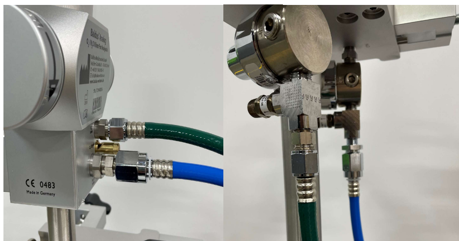
Figure 4: Attaching the Gas Hoses
