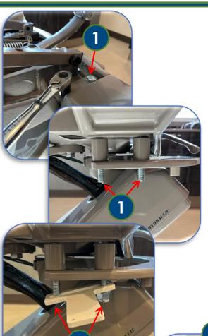
WARNING: Replace the main bolts in #1 one at a time. Do not remove both bolts at the same time.
