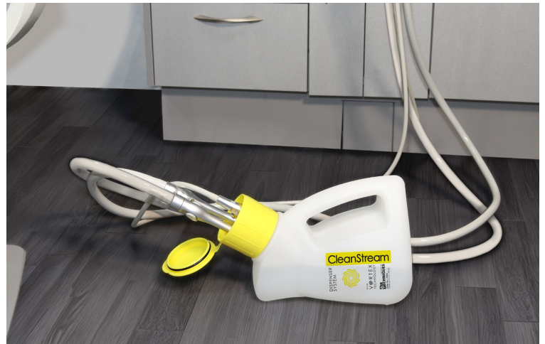
2nd operator: Turn dispenser on its side to aspirate the remaining solution.
