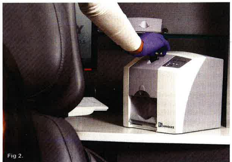
Fig 1. Flexible phosphor sensors have an imaging area that is 17% to 38% larger than rigid sensors. Fig 2. Ultra-compact flexible phosphor sensor units are designed for time-saving chairside use.
